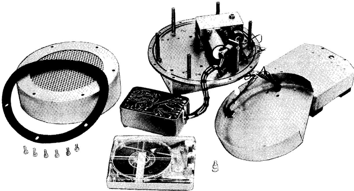
Fig. 3. The disassembled FBK. The micromotor and drive assembly is at upper center. The electronics module is in the center. The magnetic tape cartridge is at bottom. (Photo courtesy of Geodyne Division, EG&G International)
