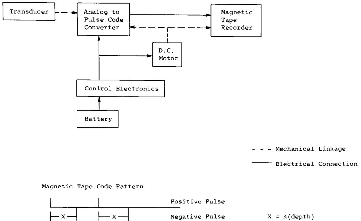
Fig. 4. Block Diagram of the Pulse Code Magnetic Tape Recording FBK.
