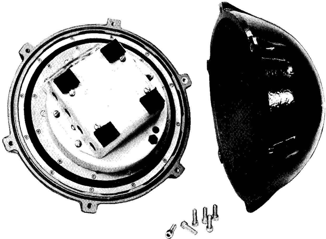
Fig. 2. View of instrument platform mounting plate group with top hemisphere removed. Battery package is visible with rubber "bumpers" at each corner. Tape cartridge partially visible upper left. Shock isolator assembly and housing O-ring can be seen in place. (Photo courtesy of Geodyne Division, EG&G International)
