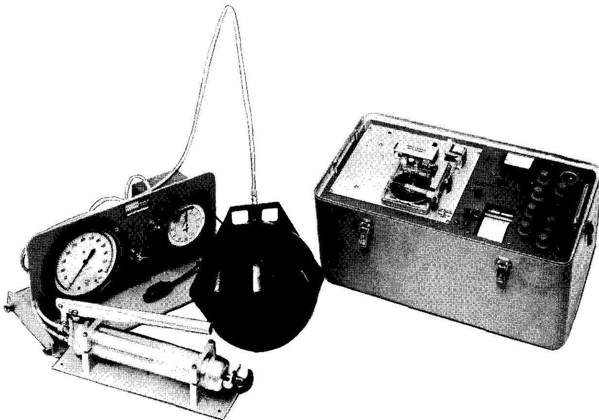
Fig. 1. The FBK and Dockside-Support Equipment. The FBK is connected to the time and pressure calibrator (left). The analog playback system is shown on the right. (Photo courtesy of Geodyne Division, EG&G International)
